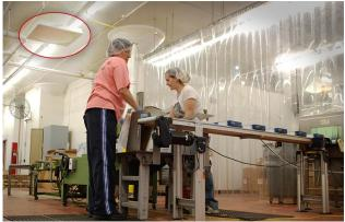
RF Controls' ceiling-mounted smart antenna panel (circled in red) is monitoring the production line. Business rules allow RF Controls' technology to count, locate and track any item moving through the line.
